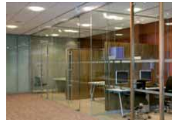
Full height single glazed Polar with veneered Workwall modules
