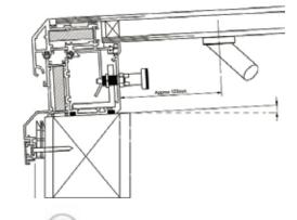
VisionVent® (Vent & Mainenance Access) Bespoke Sizes Available (up to 2m2) All sizes refer to Overall weathered upstand dimensions
