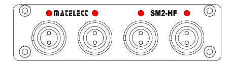
Figure 4. Front panel of SM2-HF
