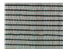
Cross-weave; Filaments along length and across width of tape
