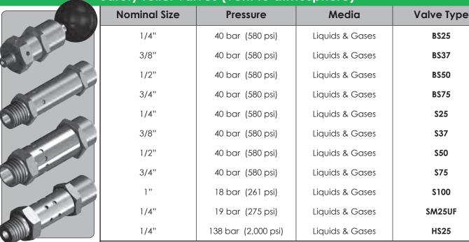
Safety relief valves with a vent to atmosphere feature, stainless steel construction (BS variants in Brass). Valve designs mostly incorporate elastomeric sealing technology for virtually zero leakage performance. Relatively high discharge capacities are achieved via the pop-open style valve characteristic. BSP and NPT inlet port options available. Not designed for use with corrosive or hazardous media.
