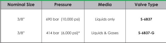
Four port directional control valves, stainless steel construction. Balanced spool technology. Service pressure does not affect switching pressures. Various actuators, port options and seal options available. \* NOTE - Pressure rating is reduced with gases
