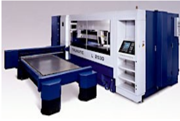
One Trumf L2530 plus 4kw Laser, 2500mm x 1250mm cutting area.
