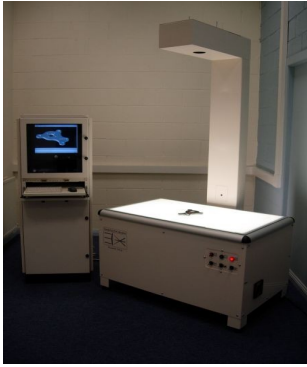
Inspecvision Laser based coordinate measuring system
