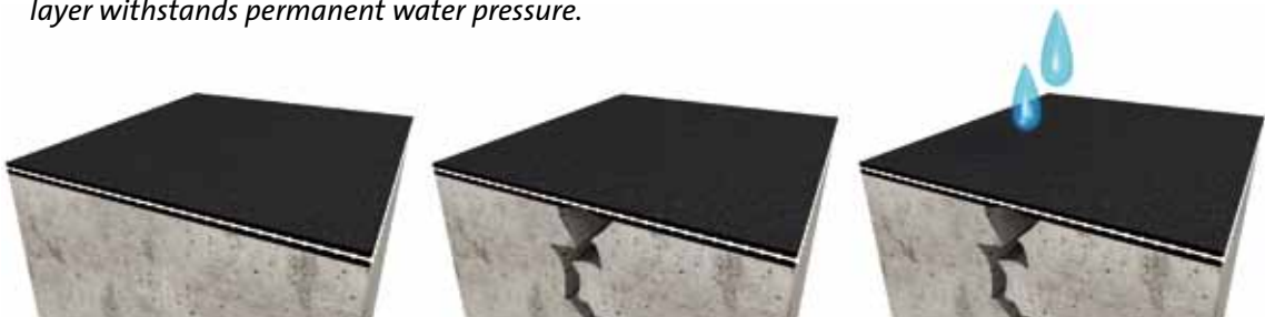
3. Crack bridging due to an embedded mesh. The mesh separates the top waterproofing layer from the crack and helps significantly to withstand permanent water pressure.
