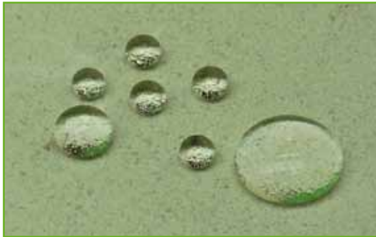
Hydrophobing : Making the building material water repellent
