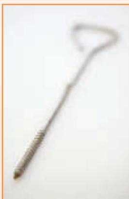
Stainless Starter Ties can be screwed directly into door and window frames to join them to new brickwork, alternatively sizes 150mm and above have a drip feature for use where there is a cavity and a new wall needs to be built.
