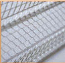
Rib Lath, stiffened by longitudinal ribs, for use on ceilings and partitions as well as walls. Stainless Steel should be used for external work or in damp conditions.
