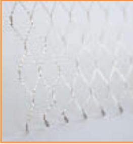
Expanded Metal Lathing is mainly used as a key for plaster when applied on suspended ceilings and walls. It is also suitable for encasing steel columns and beams, assisting in the protection of fire. Stainless Steel should be used for external work or in damp conditions.
