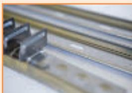
A superior Stainless Steel Wall Starter System for joining new walls to existing masonry, suitable for both internal and external brick or block walls, the connectors can be slotted together up to a maximum of 8 metres or 3 storeys high, from 60 to 250mm thick.
