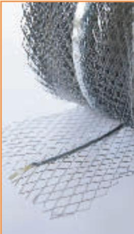
EML Brick reinforcement is primarily used to prevent cracking, reinforcing brick and block work. Stainless Steel should be used for external work or in damp conditions.
