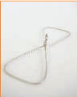
Traditional Butterfly Wall Tie previously to BS1243. The central twist must be placed down the cavity to prevent moisture travelling across the cavity.
