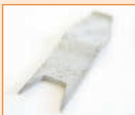
Framefast are used to tie door window frames into brickwork. No screws are required as when the spikes are driven into the timber they spread outwards creating a fishtail effect, while the curved centre and lip create an adequate mortar key.
