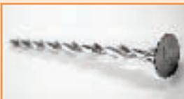
Suretwest Composite Panel Fixings are a hammer driven fixing for securing structural 6mm plywood composite insulation board to flat roofs. 20mm diameter head. Approved by the major insulation suppliers.
