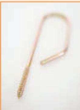
Screw tie 150mm long, to tie timber door / window frames to adjacent brickwork.
