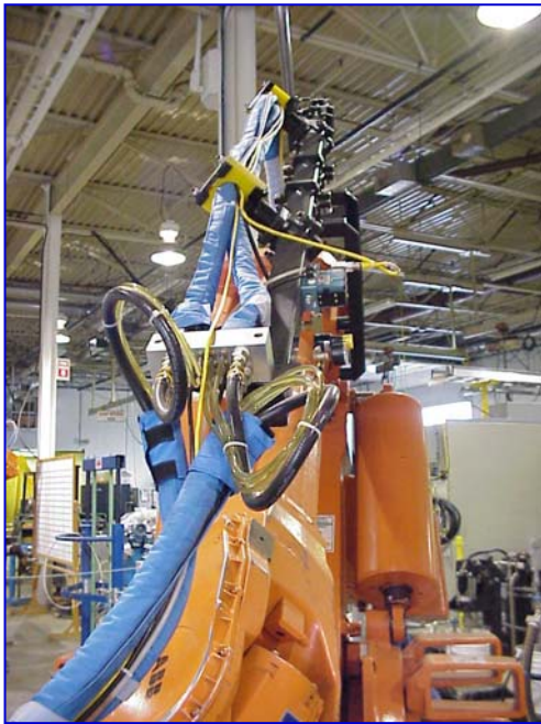
Robot Dress-Out along Robot Arm
