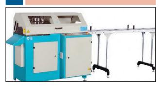
Dedicated Auto Cut System with roller side table for accurate flange cutting
