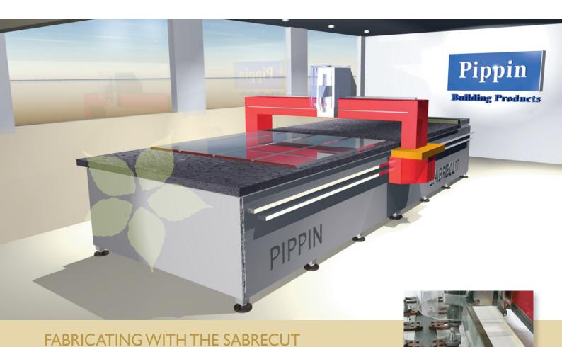
An innovative range of CNC machines that are designed specifically for the pre-insulated ductwork and insulation industry, featuring an angle cutting head that automatically pre cuts the sheets ready to easily fold into and form the ductwork component.
