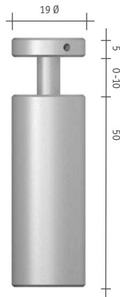
PSD.0 Panel support for drilled sheet
