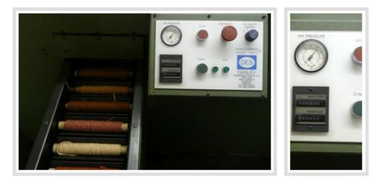
Designed for the carpet weaving and spinning industry to remove yarn from cheese centre packages. The TWS 1 Automatic yarn stripping machine removes yarn from parallel packages to a maximum capacity of 800 per hour. The operator simply loads the packages on to the conveyor tray. The yarn is stripped and directed down one chute whilst the empty package is deposited down a separate chute. The machine is guaranteed for 500,000 packages or 12 months.
