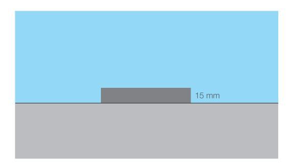
When fitting the aluminium wedge it is essential that when pressed in firmly by hand that the wedge protrudes approximately 15mm above the alloy shoe channel prior to hammering in with the lump hammer and bolster. Due to manufacturing discrepancies the size and thickness of some parts may vary, however every effort is made with quality control checks. We have found that glass thicknesses vary up to 1mm plus or minus, and this is out of PureVista's control.
