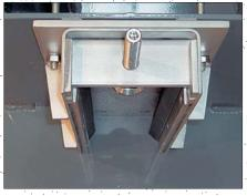
Assembly face mounted in the channel with dowels in case of large flood heights. The end posts are placed face mounted with spread anchors. Shear connectors can be used alternatively for attachment. The end posts are mounted on base plates. Gusset plates are installed between the end posts and the base plate to meet static requirements.
