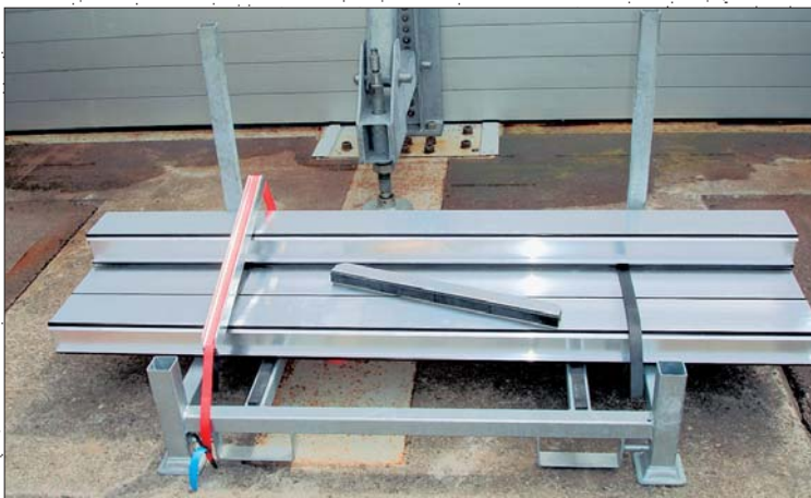
Storage rack components: Lashing strap, pressure strip, rubber spacers, base pallet frame and stanchion pipes
