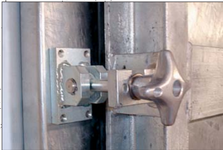
Contact pressure is achieved using two star knobs
