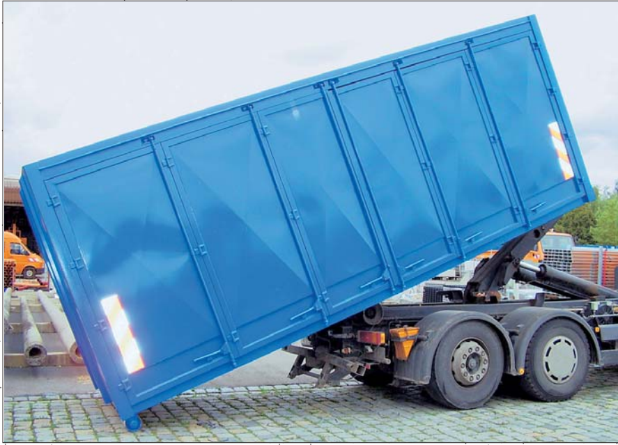
Transport container at LKW-hook being loaded
