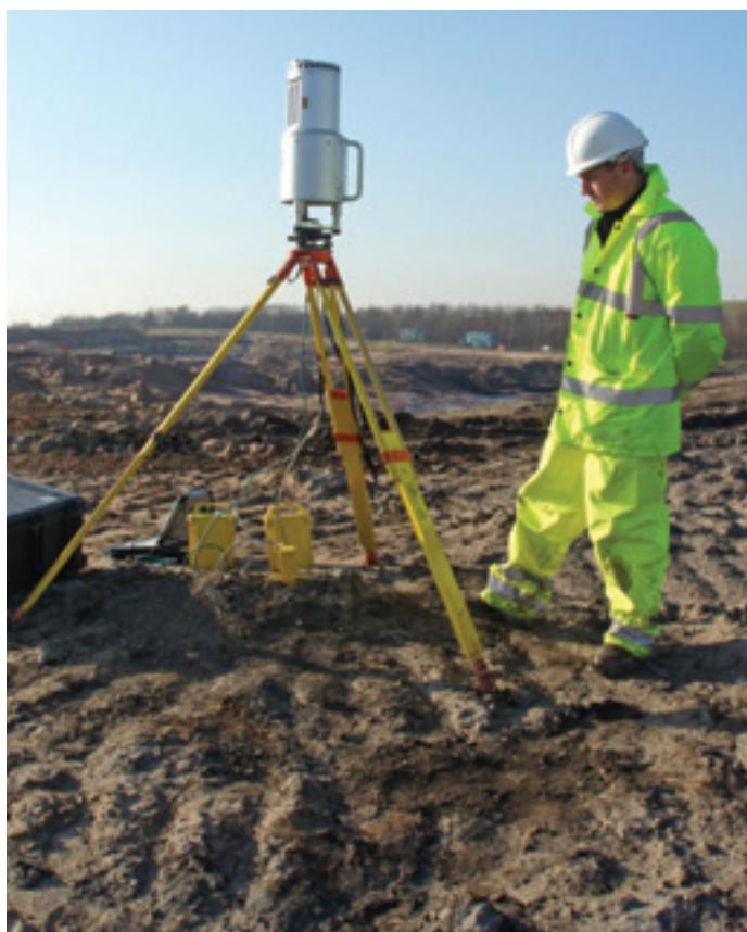
John Halifax commented, "The new Riegl LMS-Z620 will enable us to expand our operations into new areas while still maintaining the high levels of service and performance our clients have come to expect. In trials earlier this year, where we used the scanner to survey landfill sites, we were able to significantly reduce the time spent on site and survey previously inaccessible and therefore un-surveyed areas."
