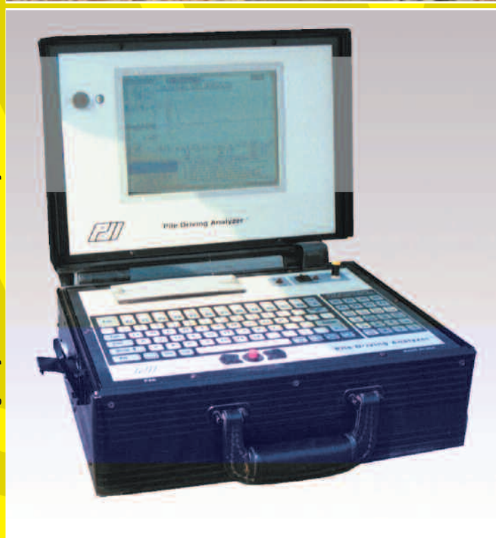
Pile driving analyser for collection and analysis of test data
