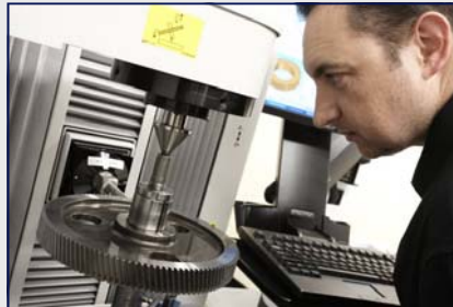
New Gleason 350GMS Gear checking machine
