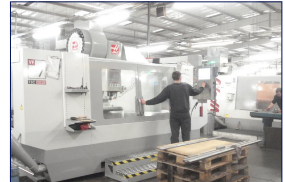
CNC Rack Milling & Drilling Including steering racks for cars
