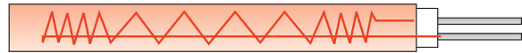
Anfang und/oder Ende st"rker beheizt Reinforced power distribution on one or both ends
