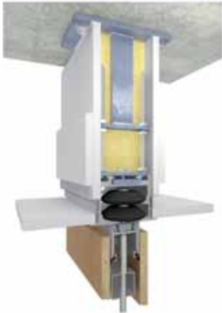
ACOUSTIC BARRIER TYPE 2 FOR VALUES UP TO R_w 48 dB
