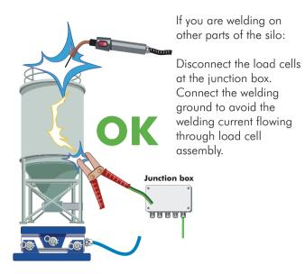
Protect the load cell assembly from splatter, overheating, and mechanical overload.
