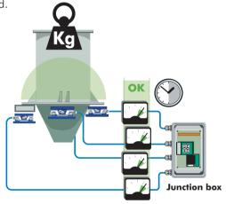
When the system is correctly shimmed, the millivolts output from each load cell will be within 20% of each other, and the signal should be stable.
