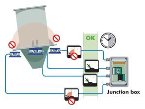
If the load cell outputs differ by more than 20%, shim plates should be fitted to level the system. Shim plates should be positioned between the top plate of the load cell assembly and the foot of the vessel.
