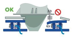
Apply a known load. Again measure the output from each load cell. Ensure that each output is still within 20%. Inspect the installation and add further fine shims as required.
