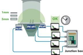
Shim plates can range from 1mm to 5mm thickness. 1mm should be used for fine shimming. Take care where shims are positioned. Shims must cover the full area of the load cell plate, evenly distributing the force.
