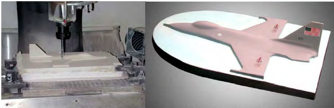
Figure 11. An F-16 replica machined from a block of paste-based tooling material
