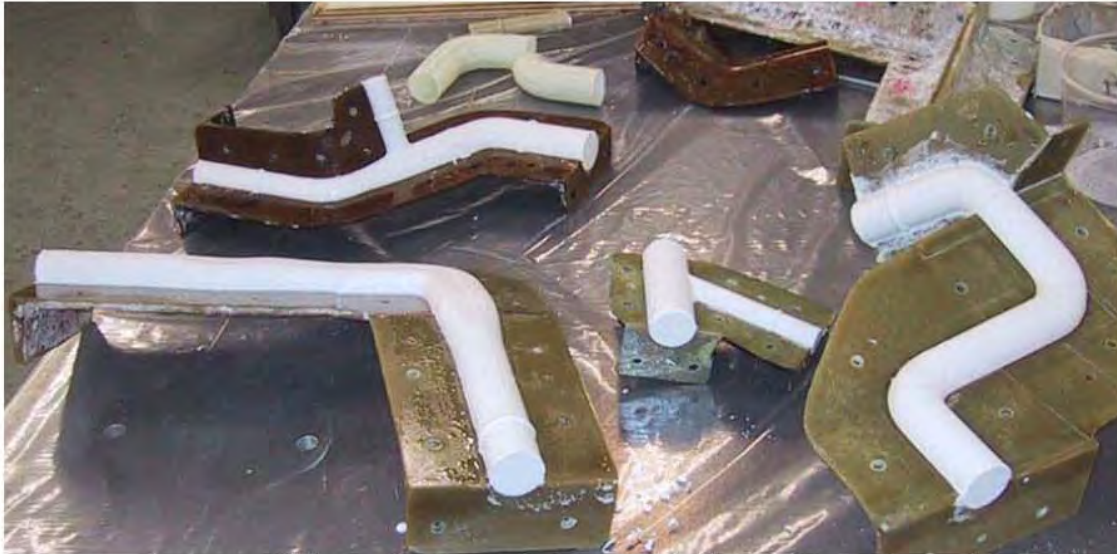
Figure 6. Different ducting tool pieces made from a composite mold
