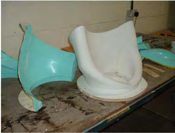
Figure 7. Tool for an inlet duct
