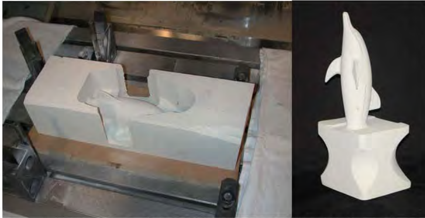
Figure 10. A complex-geometry part being machined from a block of paste-based tooling material
