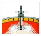
Cardox consists of a high strength reusable steel tube filled with a liquid carbon dioxide, a chemical heater and a rupture disc. When energised by the application of a small electrical charge, the chemical heater instantly converts the liquid carbon dioxide to a gas. This conversation expands the CO2 volume and builds up pressure inside the tube to burst. This releases the CO2 - now 600 times the original volume - through a special discharge nozzle to create a powerful
