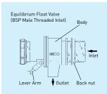
The range of EBCO high flow rate Float Valves are simple and robust and can reliably self-compensate for changes in water supply pressures. One size of seat and one size of ball float will suit any working pressure up to the maximum recommendation of 10bar (150psi) for the reduced bore float valve or 5bar (72psi) for the full bore float valve.
