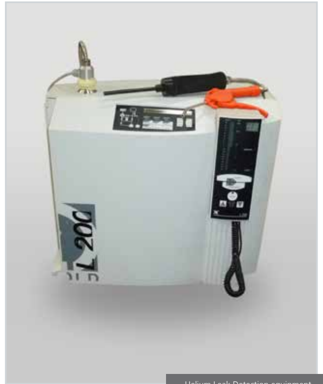
Helium Leak Detection equipment
