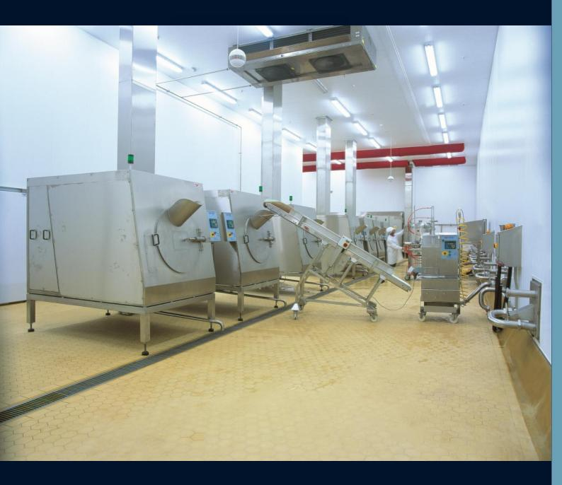
DCN cooling systems offer process innovation and excellence with minimum batch times. Cooking and Cooling is often part of the same package; a tumble chiller is part of the cook-chill system, and for processes requiring large batch cooling in stand alone vessels DCN offer an extensive range of static D A coolers with unique scraped surface agitators.
