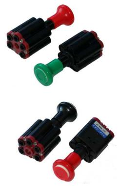
**The Manual Air Release (AR)** The AR valves require the reset signal to be removed/disengaged from the reset port before the valve may be operated and are ideal for interlocking with hand-brake air systems for additional safety. The valve may also be used as a 4/2 valve when no reset signal is required.
