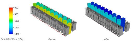
CFD simulation enabled Dell engineers to visualize bypass airflow and redirect the air to the cold aisles.
