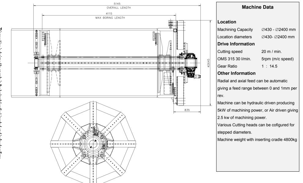
This machine is designed to operate in the horizontal, vertical, inverted, and inclined positions. The range of Reekie Machine tools cover machining capacities from zero to 10m diameter.and operate successfully on all terrous and non-terrous materials capable of normal machining
