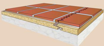
If a joint between wooden boards of a floating floor is not correctly located or fixed, it will be susceptible to highly localised movement which will crack the tile along
