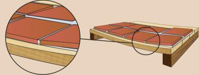
If the bed is too thin a cement-based adhesive may dry out very quickly and not gain strength.
