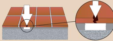
Ceramic tiles are inherently brittle and therefore any area of the tile that is not fully supported is vulnerable when subjected to a localised load. Examples could be: a chair leg, something being dropped, or any heavy item on small feet such as a kitchen appliance.
