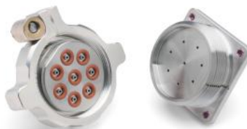
SQDC-R-8-77-S (8 way SQDC for 1mm SS tubing with silicone seals)
