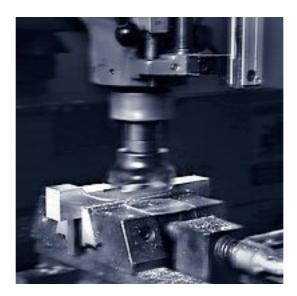
Most of our work is done on fully-enclosed wet-running machines operating automatically, but for one-off or short-run prototyping, modification and finishing jobs where step-by-step manual control is needed, we have a Bridgeport Series 1 EZ-Trak semi-automatic CNC milling machine which can be run with or without lubricant.
