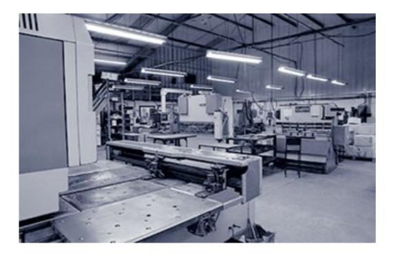
Our sheet metal operations are based on CNC machines for cutting, punching and folding.
