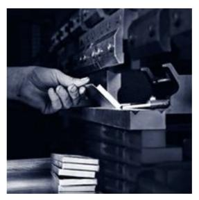
Blanks are guillotined from the sheet and a variety of punching machines are used, ranging from the fully automatic Nisshimbo 26-station turret punch press to small manual punches which are sometimes used for fine operations on small parts.
