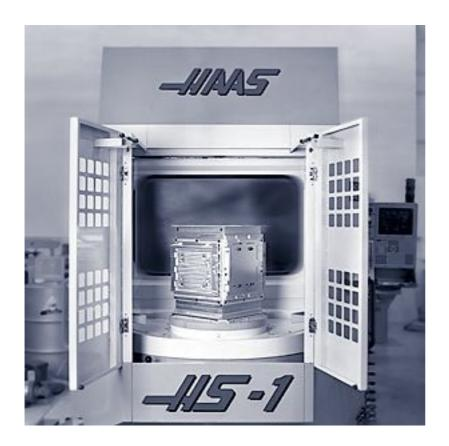
Paragon's largest machines are horizontal and vertical machining centres, the Haas HS1 and VF8. These machines are extremely versatile, allowing us to make production runs of components cut in sets from single blanks as well as giving us the capacity to make parts which would have traditionally involved a slow, expensive combination of castings and machining.
