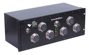
The new MIL series RACKtangle provides 12 I/O slots and uses standard DNR-series I/O boards (e.g. DNR-AI-217). It is available in the standard PowerDNR configuration or as a UEIPAC or UEISIM.
