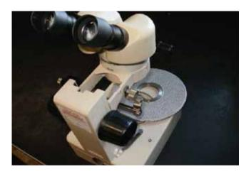
Visual Inspection - All parts processed at PPSL undergo a visual inspection regime. Parts are visually inspected both on receipt, during processing and after cleaning to look for contamination, damage and item integrity.
