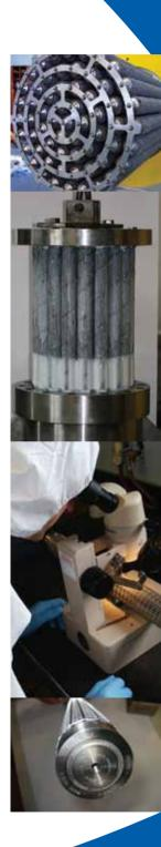
DP Testing - is a test for filters based on measuring the ratio of differential pressure across the filter to the flow of fluid passing through the filter. This measurement is a common factor in the specification of filters and the results obtained in this test can give an indication of the level of free flow in the filter.
