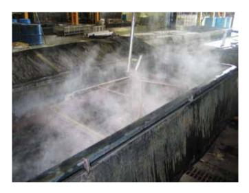
Water Washing - involves low pressure washing to provide a mechanical flushing of the parts to remove contamination and to remove cleaning chemicals.
