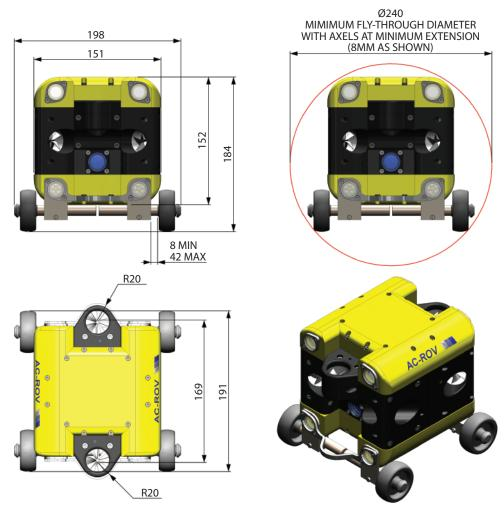
The individual rollers attach via the AC-ROV light ports, of which there are 8 in total.
