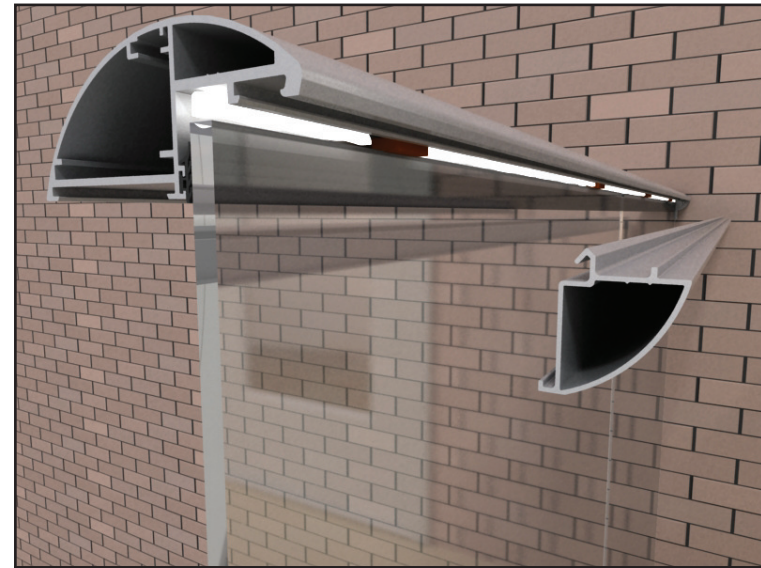
62 Replace the full length glazing beads
