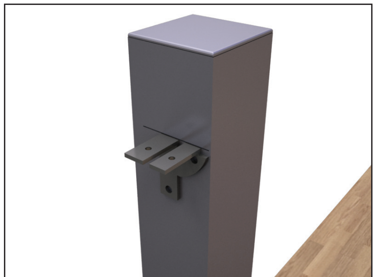
16 Bring the fixing bracket in place
