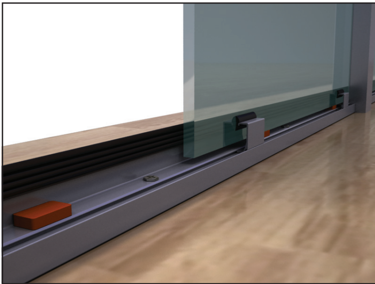
37 Use 3mm rubber gaskets to hold the glass against the small bead pieces on the bottom rail
