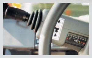
The Powershift gearbox with electronic gear selector optimises cycle times.
