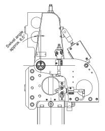
The tool is pushed against the workpiece by the swivel pedestal. Position and part tolerances are equalized, which proves advantageous for the process quality of clinching, embossing and marking operations.
