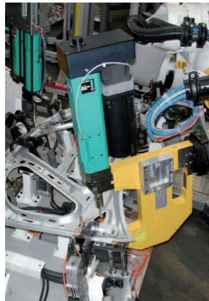
TOX®-Robot-Machine Mount Tongs with compensating slides
