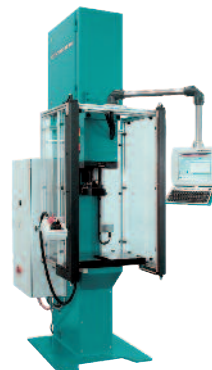
Complete press with safety control according safety level 4
