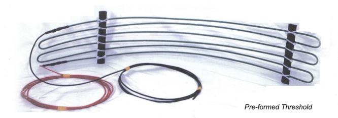
Ramp Heating systems are made of high quality heavy gauge stainless steel wire extruded with PVC and low voltage transformer. They are designed and manufactured by Thermatek for safety and efficiency in running to ensure that any coldstore ramp will be free of ice or frost and accessible to traffic at all times.
