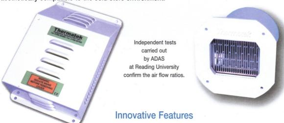
Large aperture for air flow - Valve heated to prevent icing. - Front cover moulded ABS with main body of aluminium and Stainless steel - no rust or paint can fall within the coldroom. Electrical connection to rear of valve outside the room. Valve body adhered to moulded front to allow condensation to drain away. Simple to install. 'O' ring seal to coldroom wall. Steel painted external cover over electrical connections. To be located at a height suitable for routine maintenance.
