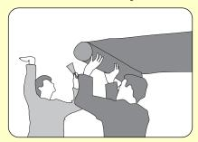
Application of the paper requires two people. One applies the CA/N adhesive at a coverage of 3m² per litre, whilst the other unrolls the paper and then presses it flat onto the surface using a standard decorator's scraper or rubber roller. Each sheet must overlap the next by 10mm to 15mm. The edges must be trimmed using a sharp knife and a straight edge, then butted together. Apply extra adhesive under the trimmed straight edges and press them flat to finish.
