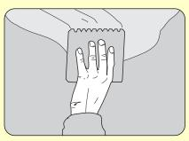
Once the surface has been properly prepared, liberally apply the adhesive (in areas of one square metre at a time) over the surface with a standard comb.
