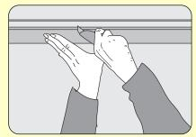
The intumescent paper and adhesive must be completely dry before decorating with either paint or paper. Treat all decorative plaster elements, such as coving and mouldings, with two coats of Envirograf® Product 105 (EP/CP) at 8m² per litre per coat. This can then be painted over with a good quality acrylic paint.
