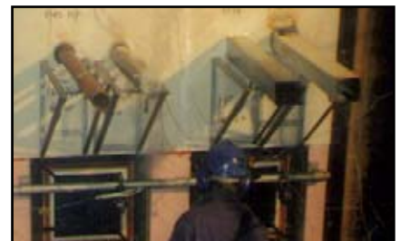
A Fireblok® sleeve applied around plastic trunking
